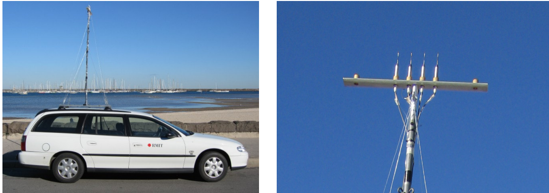
Figure 3: Cobra Probes mounted on a bracket on top of a vehicle-mounted mast.
