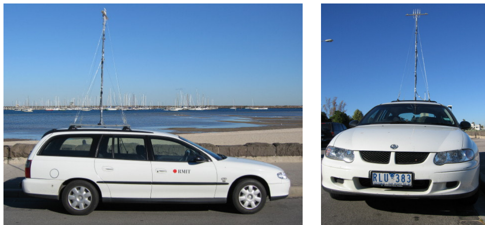
Figure 30: Mast and probes mounted to the RMIT station wagon.
