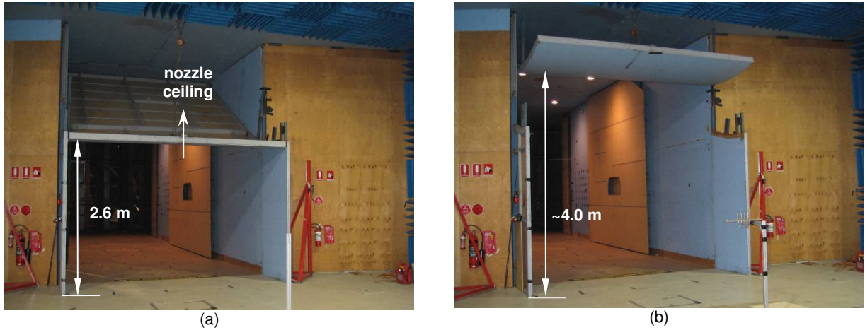
Figure 50: Photos showing changes in jet configuration, downstream of the fans, before the automotive test section: (a) jet down, standard automotive configuration; (b) jet up, wind engineering configuration.
